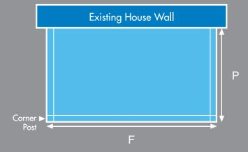
'F' front frame width (including corner posts) 'P' projection (this is measured from face of back wall to external face of front frame)
