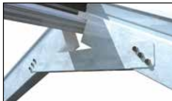
Where the eaves beam sits against the host masonry wall, it has a structural moulding attached to the eaves beam. This has three fixing positions cast into it to allow attachment into masonry – choose the hole that directly lines up with solid masonry and attach using one resin anchor suitable for substrate / loads (not supplied, see p21 Appendix 1).
