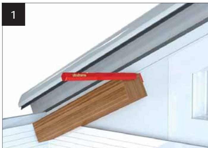
Using the location plan provided find the dimension for setting out the clip positions for the gable brackets. Measure up the bar from top edge of the fascia board and mark it.
