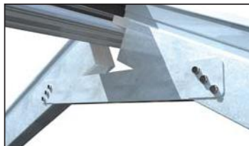
Where the eaves beam sits against the host masonry wall, it has a structural moulding attached to the eaves beam. This has three fixing positions cast into it to allow attachment into masonry – choose the hole that directly lines up with solid masonry and attach using one resin anchor suitable for substrate / loads (not supplied, see Appendix 1)
