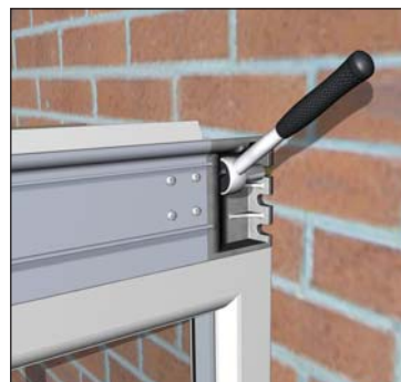
Where the eaves beam sits against the host masonry wall, it has a structural moulding attached to the eaves beam. This has three fixing positions cast into it to allow attachment into masonry – choose the hole that directly lines up with solid masonry and attach using one resin anchor suitable for substrate / loads (not supplied, see Appendix 1)
