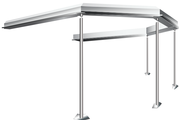
Figure 26: - Example of structural steel posts with ring-beam
