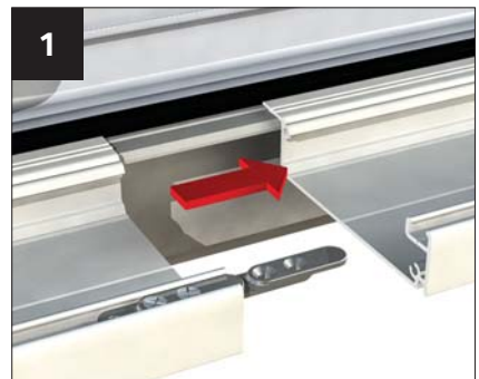
Attach the cleat CRN001 using 2 x CRN006 provided, on each side of the joint. Repeat as per image.
