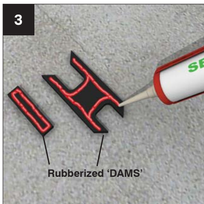
3 Take 'rubberized' sealer strips and generously butter with silicone.
