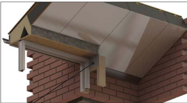
Abutment bracket is fixed to the infill timbers, angled panel bracket fixes to the wall.
