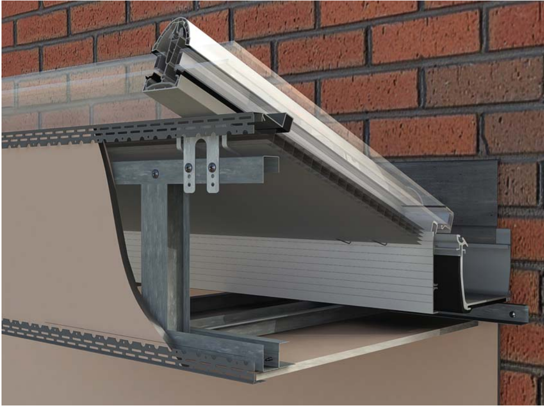
Framework terminates on host wall.
