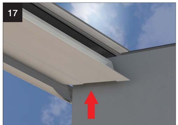
Classic Plus Valley cladding being fitted against LivingRoom . After plasterboard and skim.
